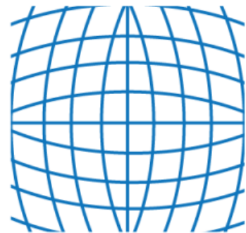
positive radial distortion "barrel"
